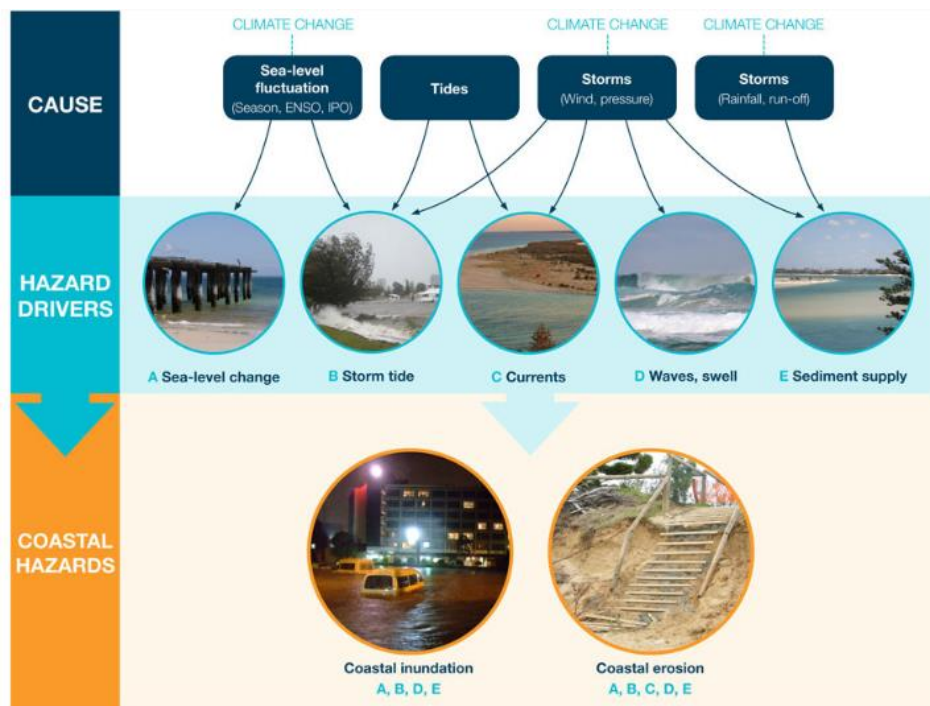
Figure 4-1 Coastal inundation and coastal erosion arise from intricate interactions between several drivers. Source: Adapted from New Zealand Ministry for the Environment 2004
