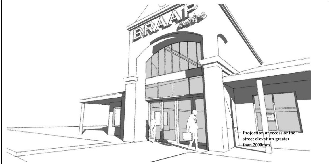
Figure 2: Building with an articulated street elevation incorporating projections or recesses of two metres or more
