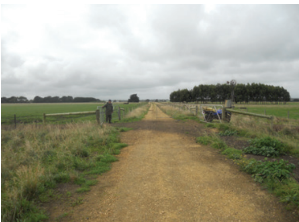
Cattle crossing gates, as used on the Port Fairy Warrnambool Rail Trail in Victoria, enable adjoining farmers, and their cattle/sheep, to cross the trail whenever necessary – thereby not hindering farming practices. Gates are closed across the trail and side gates on side boundaries opened to allow stock to cross when required. This spectacle - when it occurs - is of considerable interest to trail users.
